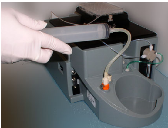
Figure B-4 Attaching the declogger tool
