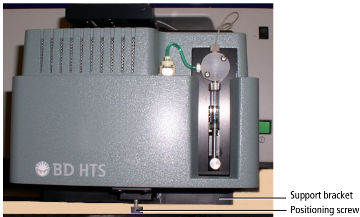
Figure 4-8 Loosening the positioning screw (example shown for BD LSR II)
