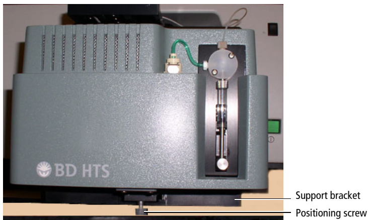
Figure 4-15 Loosening the positioning screw
