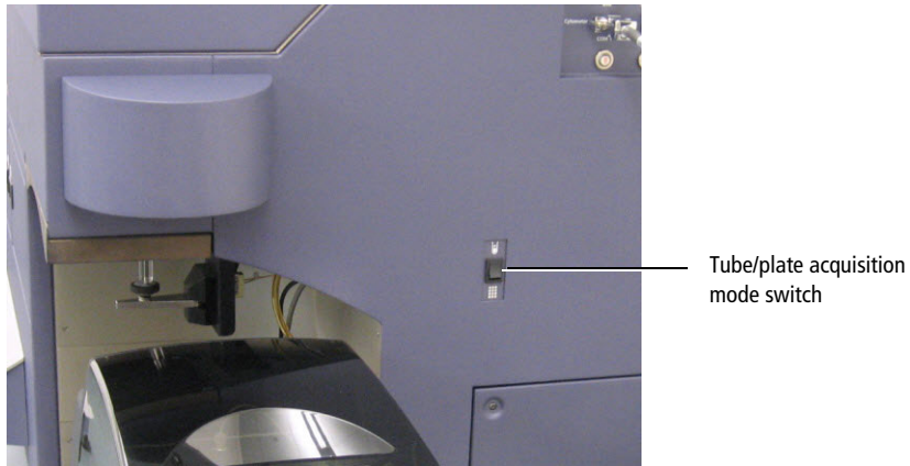
Figure 1-14 Tube/plate acquisition mode switch on the BD LSRFortessa flow cytometer
