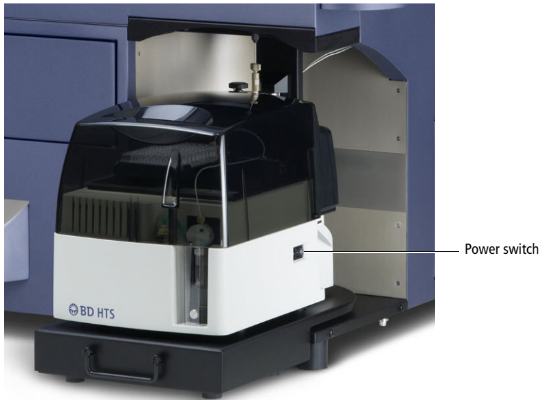
Figure 1-18 Power switch (BD LSRFortessa flow cytometer)
