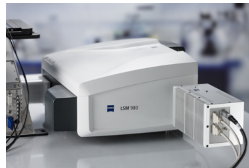
Add the BiG.2 module with its two GaAsP detectors for FCS, photon counting experiments and FLIM* to your ZEISS LSM 980.
