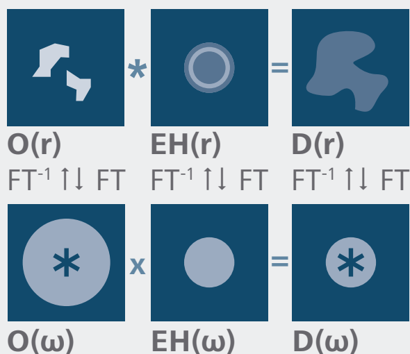
Figure B5 Image formation in a confocal system. The object O(r) in the spatial domain is convolved by the effective PSF EH(r) to obtain the Image D(r) , which will be blurred. Additionally, noise added on top of the convolution can contribute to the image (not shown). In the frequency domain, the object spectrum O(\omega) will be multiplied with the effective optical transfer function EH(\omega) to yield the image spectrum D(\omega) . Spatial domain and frequency domain can be obtained from one another by Fourier transformation (FT) or reverse Fourier transformation ( FT^{-1} ).
