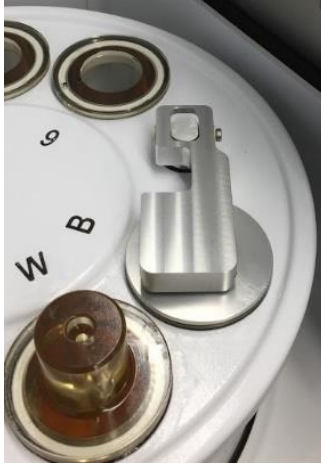
Figure 20. QC Bead Station labeled "B" Wash Station labeled "W"
