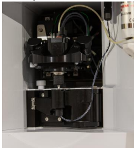
Figure 26. Nozzle in unclog/storage position
