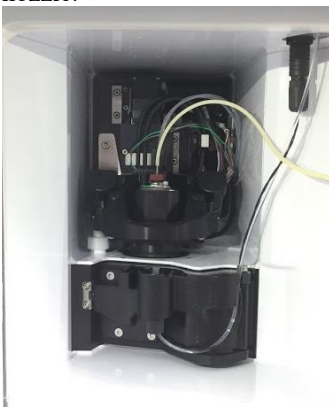
Figure 4. Behind the Nozzle Access Door, is the Nozzle and Laser Interrogation Door
