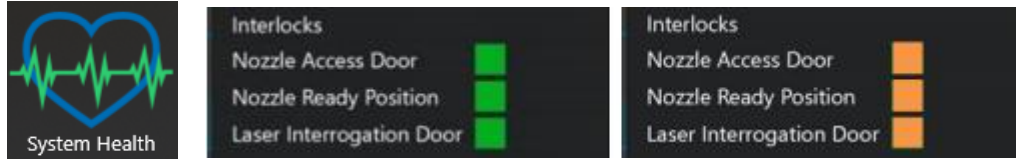
Figure 5. System Health, interlocks status green = safe, interlock status orange = not engaged
